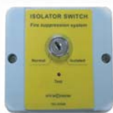
Double Pole, Key Operated, Isolator. For isolation before entry
